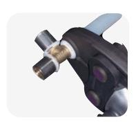
3) With the Press fittings (ROMAPRESS - RF), the pipe should be inserted in the press fitting until the end of the pipe and then press with specific tool as shown in the image. In this case, the isolating ring is used to check if the pipe is correctly introduced in the fitting.
