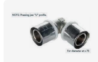
The fitting is made up of two brass parts: an 'O' ring in EPDM, a catch for the 'O' ring, a compression ring and a stainless steel interior, which confers greater robustness to the pipe/fitting transition area.
