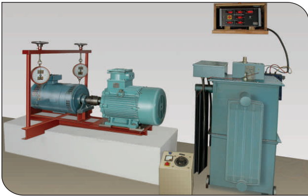
Dynamometer setup for Electric motor type testing
