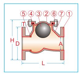
\* This length is without lining. With lining, total length shall be 6-12mm more and flange thickness 3-6mm more depending on lining thickness.
